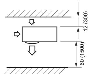
**Figure 6. Minimum operating clearances for a multiple-unit installation**
