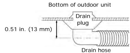
1. Insert the drain connector into the drain hole on the underside of the outdoor unit.
