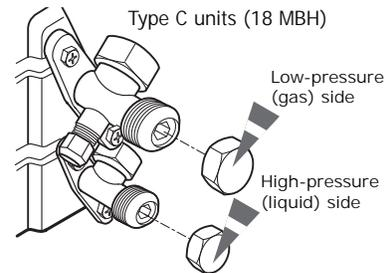
2. Close the gas side service valve, connect a manifold gauge to the valve, and open the valve again.
