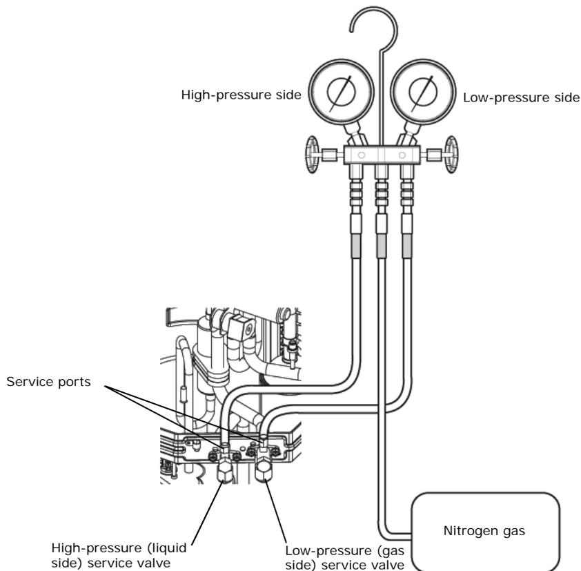
2. Fill the lines with nitrogen to no more than 594.6 psi (4.1 MPa).
