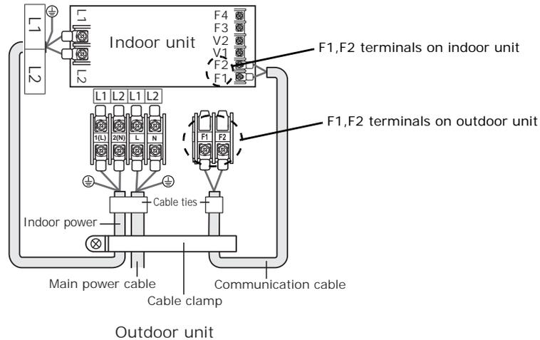
2. Provide strain relief for the communications cable.
