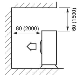
When top of unit is blocked and the air outlet is opposite the wall
