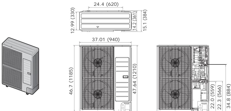
Table 3. Dimensions and weights for 18 MBH capacity units (Type C)
