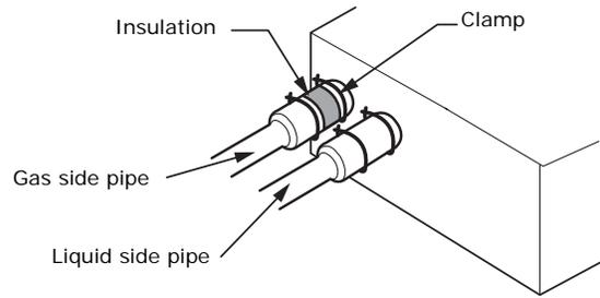
4. Cut off excess insulation.
