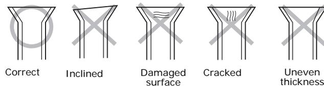
6. Align the pipes and tighten the flare nuts manually and then with a spanner torque wrench, applying the torque according to pipe dimensions:
