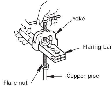
5. Remove the pipe. The end of the pipe that you flared should look like the end of a trumpet. See examples of correctly and incorrectly flared pipes.
