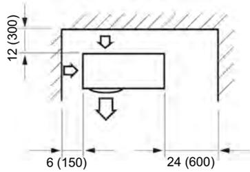
Top of unit is blocked and the air outlet is toward a wall
