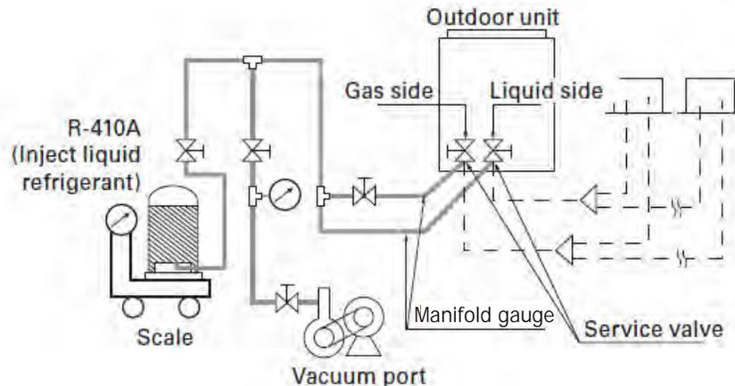
4. Open the outdoor unit service valves to release the charge from the outdoor unit.
