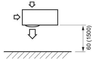
When three sides are blocked by a wall
